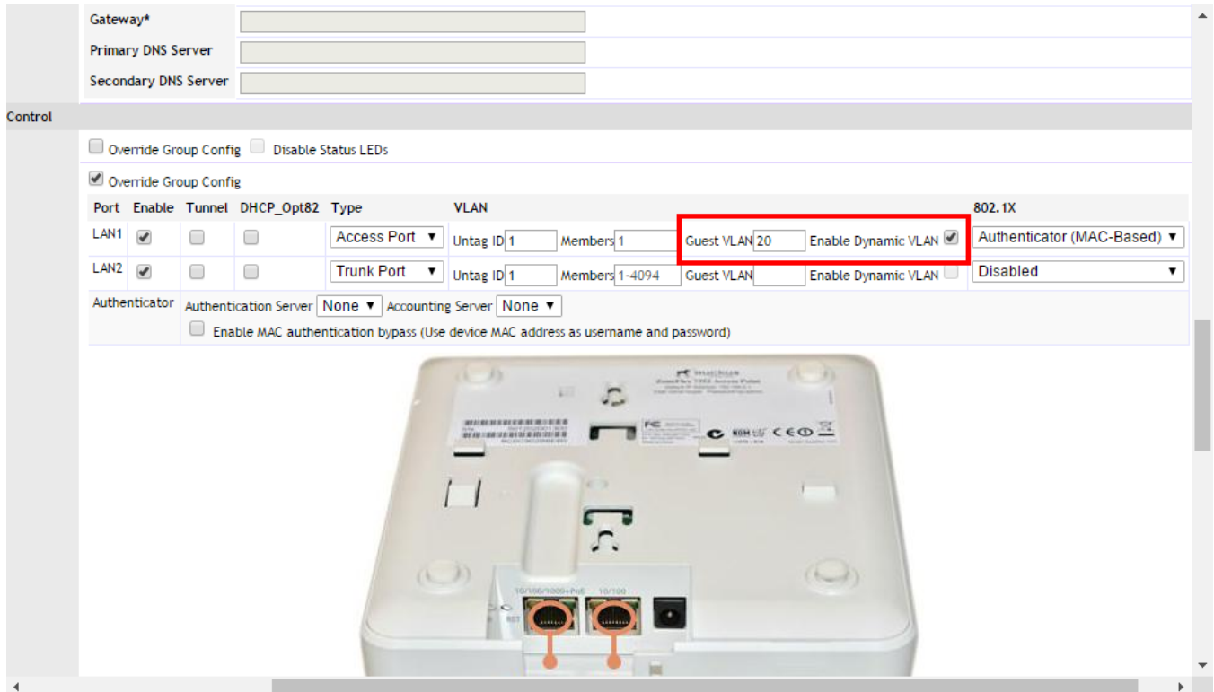
FIGURE 21 Enabling Guest VLAN and Dynamic VLAN on a MAC-based 802.1X Authenticator port
